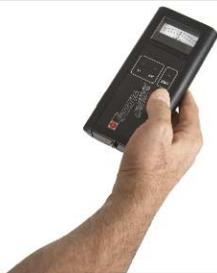
Hand Held Static Meter Model 80302 - used to indicate static charge on parts, sheets and webs. The Hand Held "Static Control" meter is reasonably priced and easy to handle. It is operated using an ON/OFF soft key (with circuit-breaker) and two further soft keys for the 0-100 and 0-1000 kV/m measuring ranges. The meter is battery powered. It should be part of any basic equipment of every electrical engineering workshop. It is rugged and durable for use in all types of plants operations.
