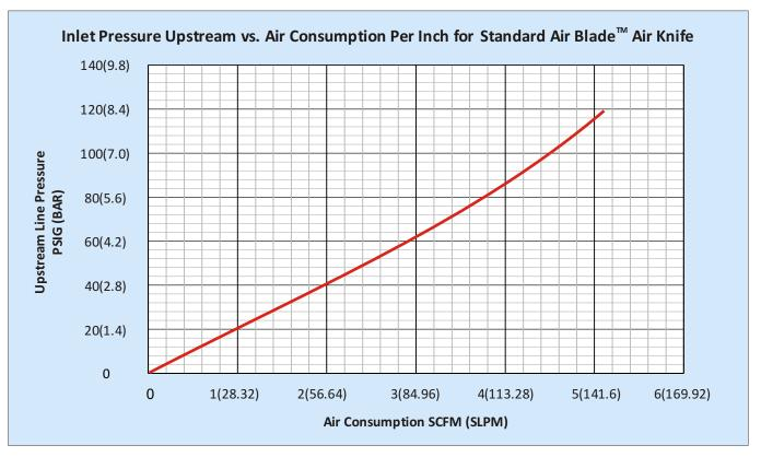
NOTE: Tests were preformed using a 12" Model 10012 Standard Air Blade<sup>™</sup> Air Knife
