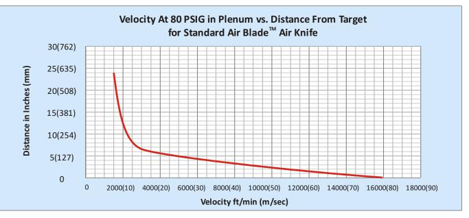
NOTE: Tests were preformed using a 12" Model 10012 Standard Air Blade<sup>™</sup> Air Knife
