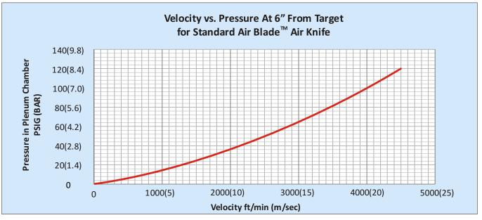
**NOTE:** Tests were preformed using a 12" Model 10012 Standard Air Blade<sup>™</sup> Air Knife
