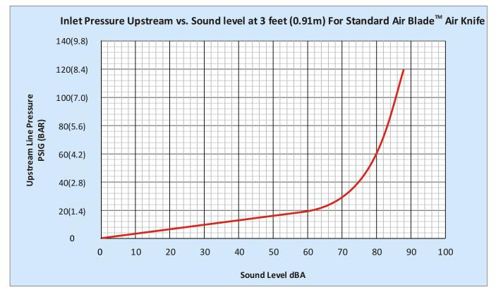
**NOTE:** Tests were preformed using a 12" Model 10012 Standard Air Blade<sup>TM</sup> Air Knife
