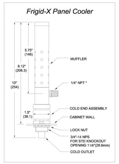
4. A cold air distribution hose kit is provided along with the cooler free of charge to direct the cold air to any hot spots as required. Holes may be cut or drilled in the tubing. Use at least 6 – 1/8" diameter holes in the tubing to minimize any back pressure on the cooling unit. The end is typically plugged and the kit is supplied with an extra muffler at the plugged end.
